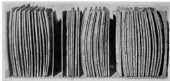
Fig. 208. An Unusually Bad Case of Buckling
