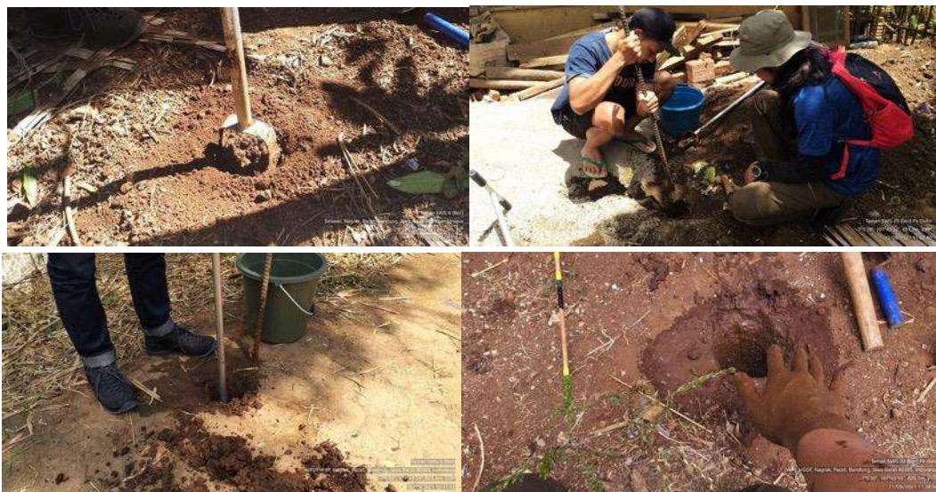
Figure 11.2 The Process of Making Percolation Test Holes by the Team and Several Communities Helping the Itenas Team
