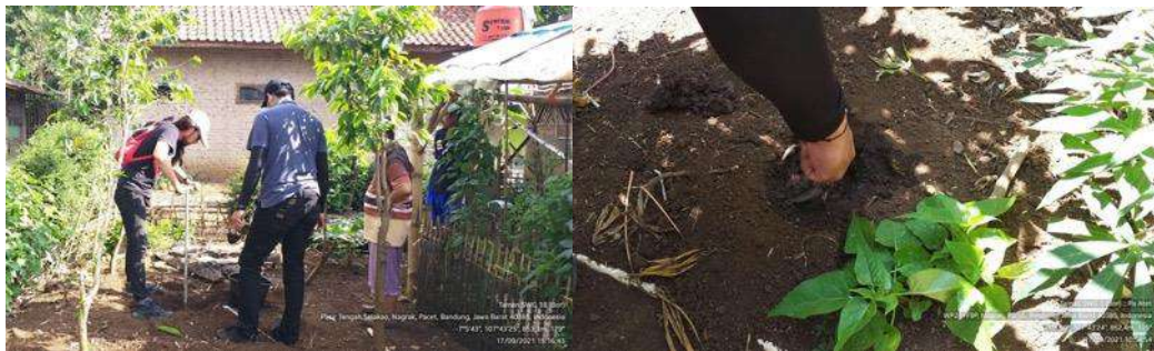
Figure 11.1 Percolation Testing at SWG Point Location
