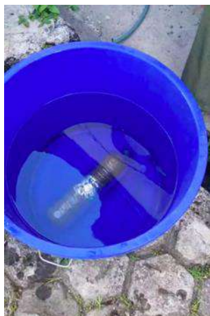
Figure 6.4 An SWB Bottle sinking in the Water – which means it passes the “sink test”!
