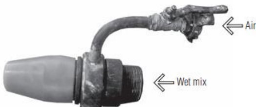
(c) Tipikal nozzle pencampuran basah hand held jenis pendek
