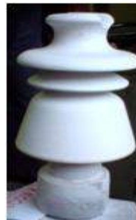
(b) Coated insulator (post pin type)
