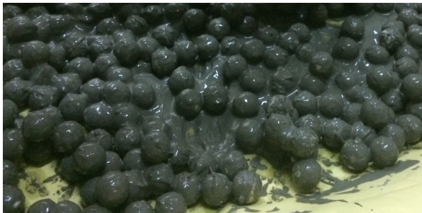
Fig. 1. Process of coating on styrofoam ball surface.
