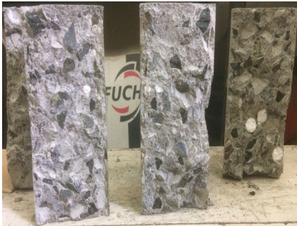
Fig. 9. Split-tensile strength test of coated styrofoam balls concrete.
