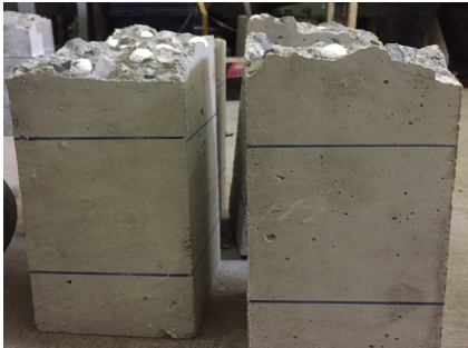
Fig. 10. Flexural strength test of coated styrofoam balls concrete.
