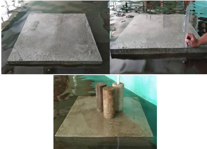
Gambar 9. Setting up benda uji pelat floating concrete
