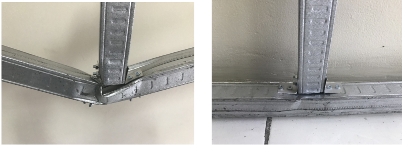
Fig. 5. Static monotonic loading test of CFS beam-to-column connections specimen 1 and 2.
