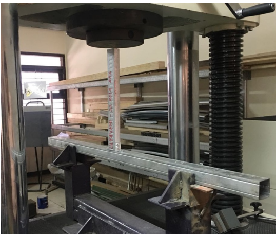
Fig. 1. Testing set-up of CFS beam to column connections.
