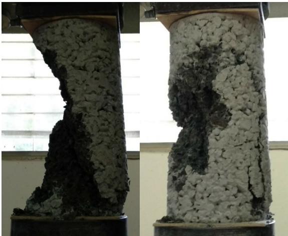
Fig. 4. Compressive strength test of porous concrete.
