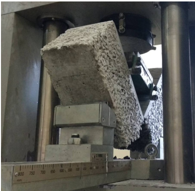
Fig. 8. Flexural strength test of porous concrete.
