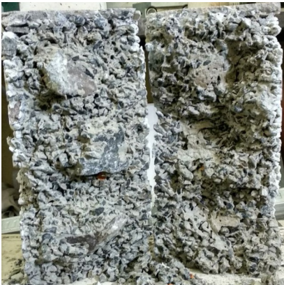
Fig. 6. Split-tensile strength test of porous concrete.
