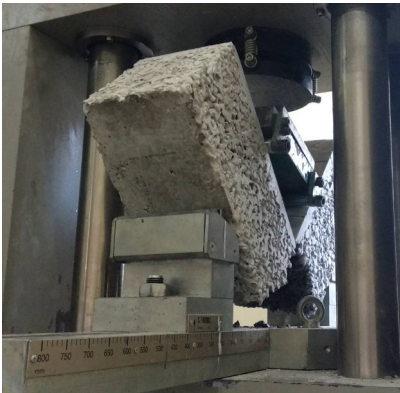
Fig. 8. Flexural strength test of porous concrete.
